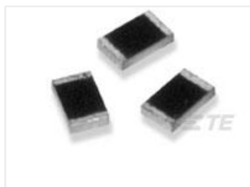
TE Part #5-1879281-9 RP 2A 487K 0.1% 15PPM 1K RL
