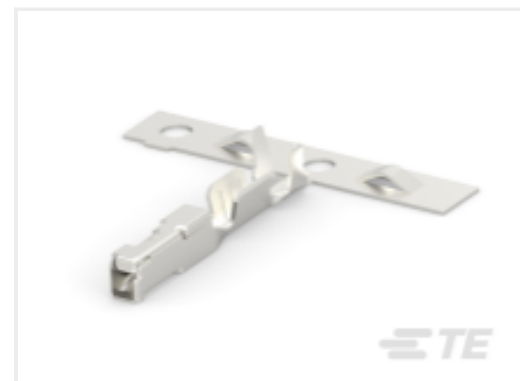
TE Part #2203242-1 Contact, female, 0.64, CuNiSi, 20-22AWG
