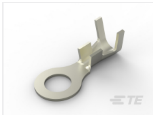
TE Part # 485003-1 RING 22-18 AWG 0.0195 X 0.5 NPST
