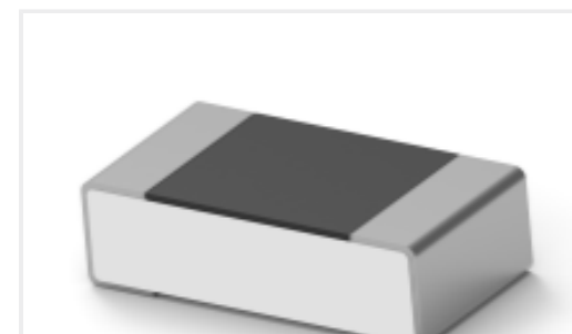
TE Part #8-2176371-3 RQ 0603 33K2 0.1% 10PPM 5K RL
