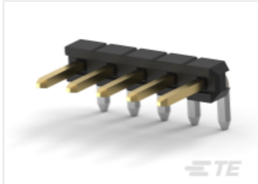
TE Part # 2842124-6 6P,2MM,BRK HDR,SRRT,2.8,0.76AU, BOX
