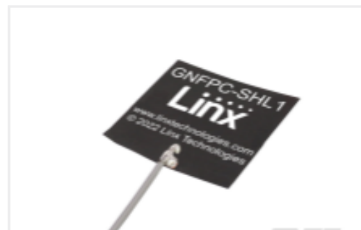
TE Part #L9000344-01 Antenna GNSS FPC SH L1 25x25 100 UFL
