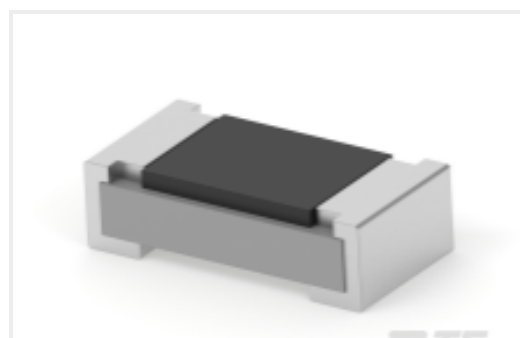
TE Part #5-2176237-0 CPF A 0603 30K 0.1% 25PPM 5K RL
