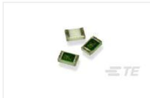
TE Part #1879337-5 CPF 0603 2K74 1% 50PPM 1K RL
