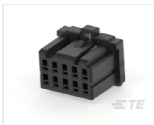
TE Part #CAT-D9934-A15B Receptacle and Tab Housing: 2.5 mm Pitch, 250V
