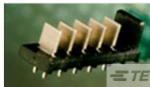
TE Part #5787444-1 HDR ASY,VERT,NO KEY,STR TAIL
