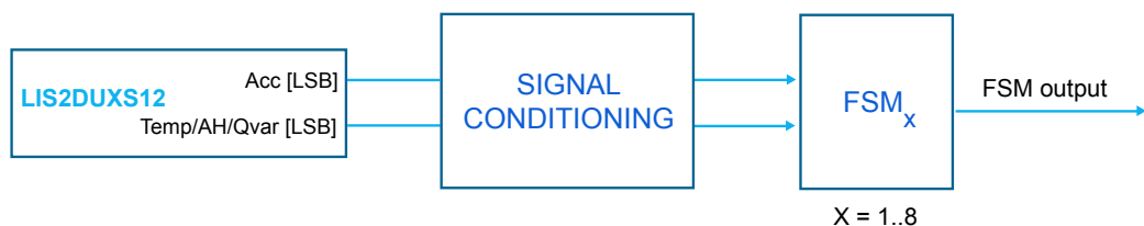
Figure 12. State machine in the LIS2DUXS12
