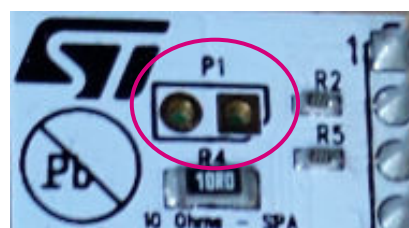
Figure 5. P1 header location
