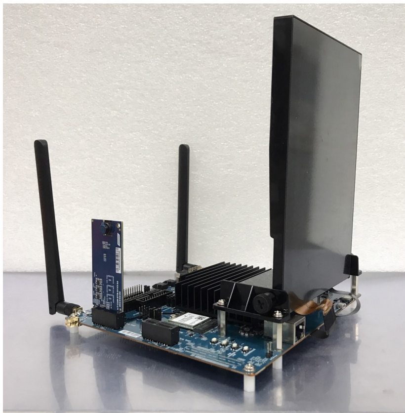
Figure 2-1. Genio 510 EVK Board System Setup
