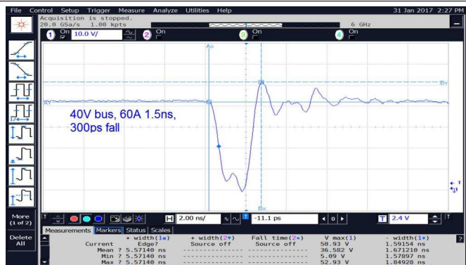
Figure 14. V_{DS} for 1.5 ns Pulse With 40V of Bus Voltage
